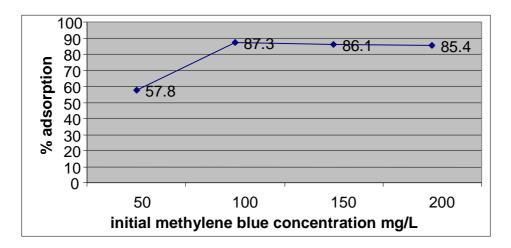
Figure6. Effect of initial methylene blue concentration on % removal
