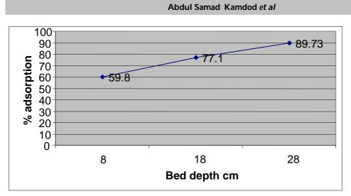
Figure8. Effect of bed depth for Cr(VI)
