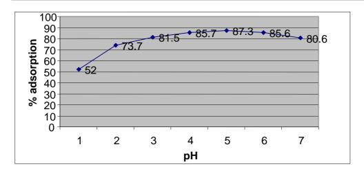
Figure3. Effect of pH on % removal of mehtylene blue
