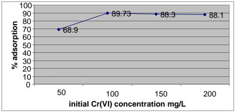
Figure5. Effect of initial Cr(VI) concentration on % removal
