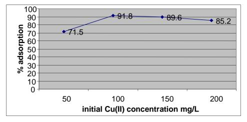
Figure4. Effect of initial Cu(II) concentration on % removal
