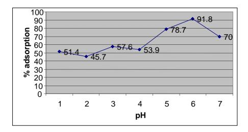
Figure 1. Effect of pH on % removal of Cu(II)
