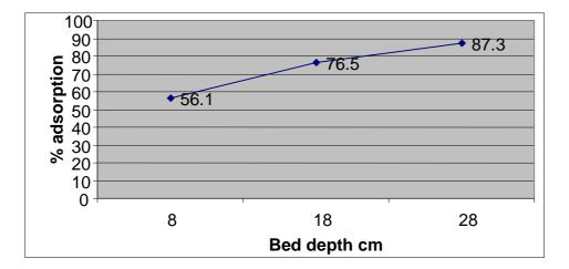
Figure9. Effect of bed depth for methylene blue
