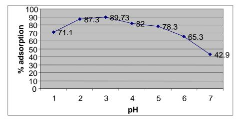
Figure 2. Effect of pH on % removal of Cr(VI)
