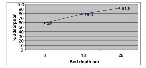
Figure 7. Effect of bed depth for Cu(II)
