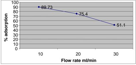
Figure11. Effect of flow rate on Cr(VI)
